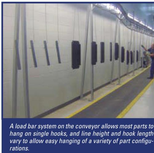
*A load bar system on the conveyor allows most parts to hang on single hooks, and line height and hook length vary to allow easy hanging of a variety of part configurations.*
