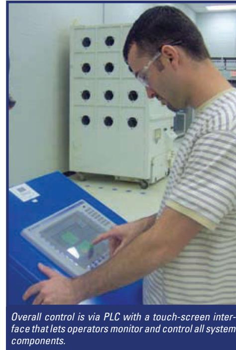
Overall control is via PLC with a touch-screen interface that lets operators monitor and control all system components.
